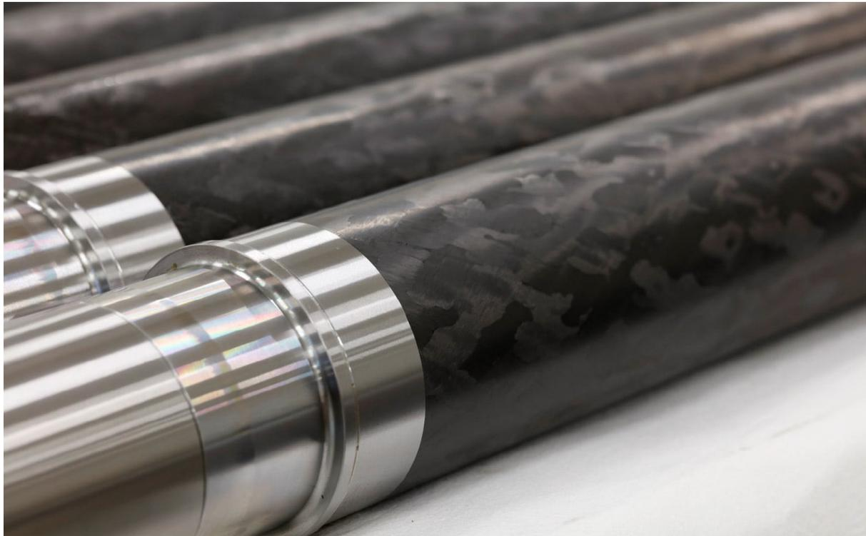
The roller, designed for paper, fabric, and nonwoven converting machines, combines high rigidity with remarkable lightness, resulting in reduced deformation even under the tension of the film running through the system. This ensures high levels of production and quality. Fibercompositi manufactures cylinders for converting, with diameters up to 300 mm and lengths up to 7 m.
